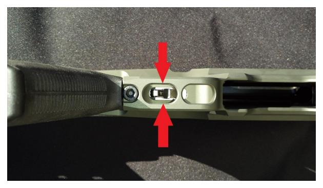
Torque both action screw – Front screw first, followed by the rear screw (55in/lb for both)
