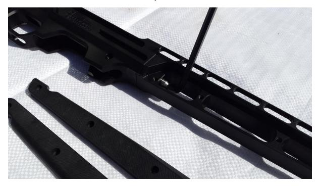
Using the 6mm Allen Key, firmly fasten to fore-end to the action block with the M8 bolt. – Be careful not to damage anodised surfaces in this process.
