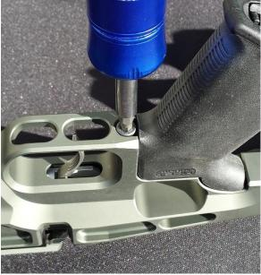
Fitting Magazine Catch – With the spring fitted to the bore of the magazine catch, insert the unit from rear engaging it forward to line up with the retaining pin.
