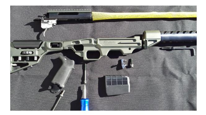
Ensure all components are clean and free of debris, in particular the bedding areas indicated below. I film of oil can be applied for corrosion protection at this stage.
