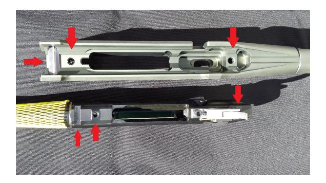
With the barrelled action sitting with the trigger assembly facing upwards, place chassis over the action carefully – Ensure the recoil lug in the stock is keyed into the action slot, the action screws of the action are lined up with corresponding bores in the chassis.
